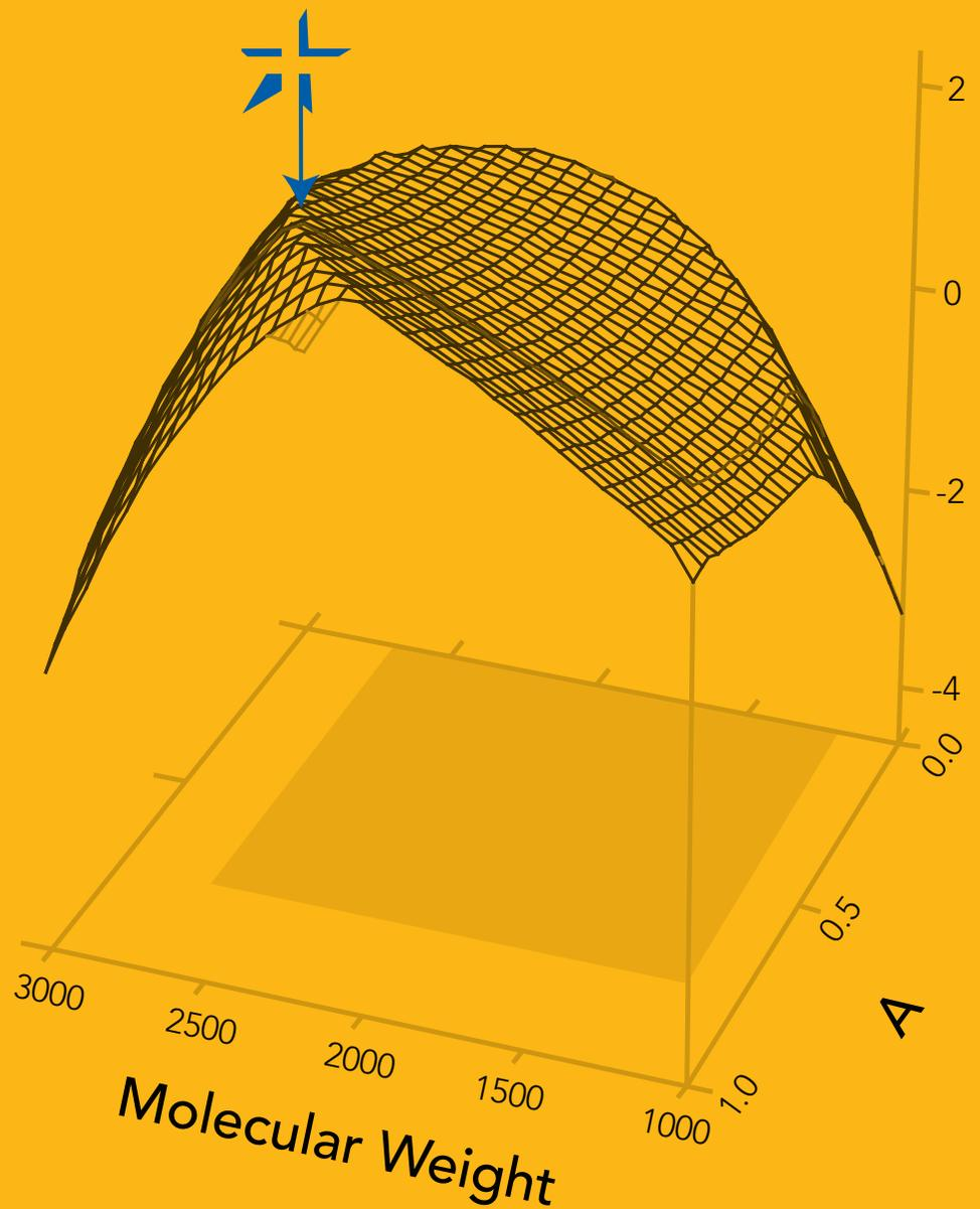
Three-dimensional Response Surface Diagrams and other models are generated as part of the Paraplex Approach. The image to the left illustrates the optimized chemical composition of a custom-designed plasticizer with the best combination of properties for the application in question. The Hallstar star next to the arrow indicates the optimal solution point.
