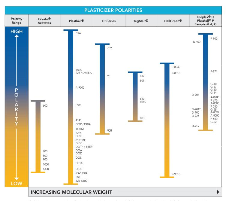
The higher a plasticizer is placed on the chart above, the higher its polarity; the further to the right of the chart, the higher its molecular weight. Plasticizer polarity does not necessarily guarantee compatibility in a polymer/formulation but can be used as a general selection guideline. Please consult a Hallstar Technical Expert for additional guidance.
